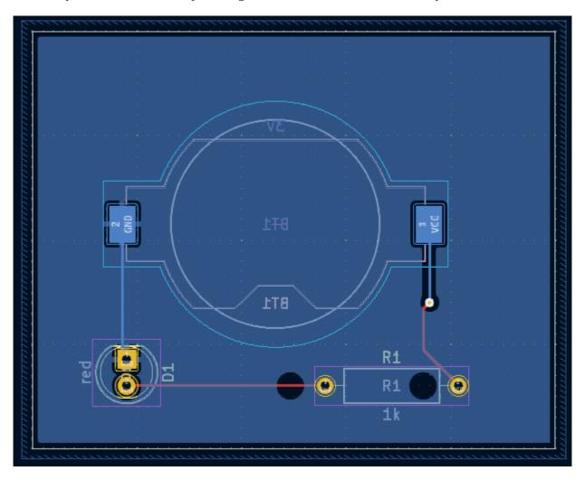
Run DRC again, but make sure to uncheck the *Refill all zones before performing DRC* checkbox. DRC reports 4 violations: for each pad of R1, there is a clearance violation between the pad and the zone and another clearance violation between the pad's through hole and the zone. Arrows point to each violation in the canvas. Clicking on each violation message zooms in on the respective violation.
