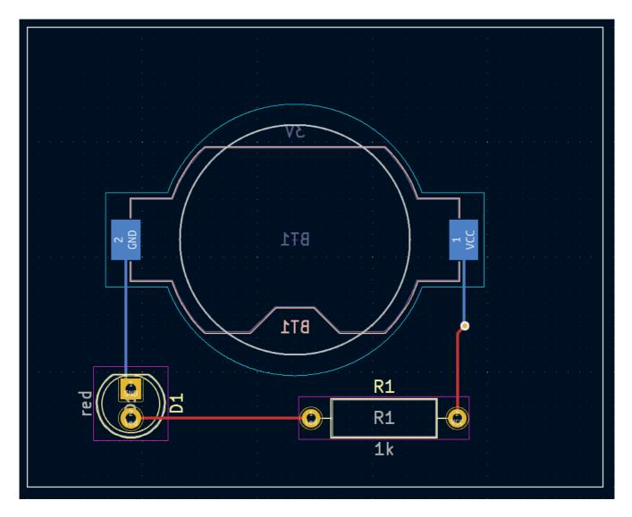
At this point, all connections are routed. This can be confirmed by looking at the status screen in the bottom left of the window, where the number of unrouted nets is given as 0.
